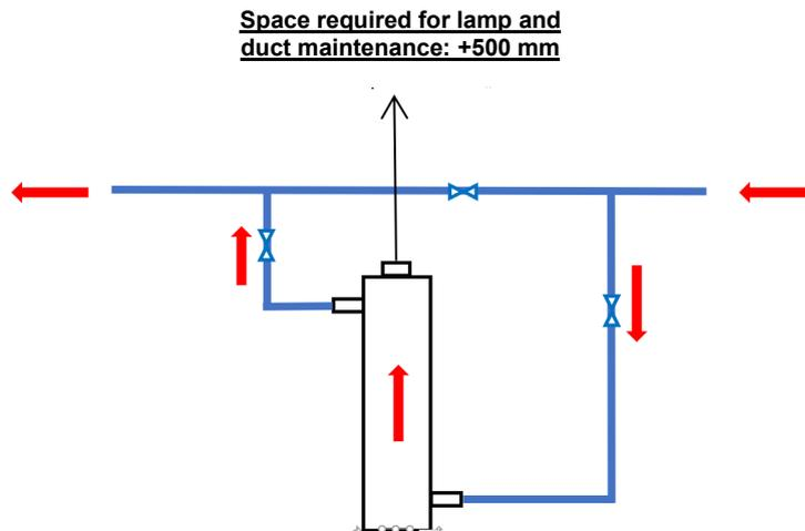
**It is imperative to always position the water inlet on the lowest tap of the reactor => filling by low point, outlet by high point, to evacuate air accumulations**
