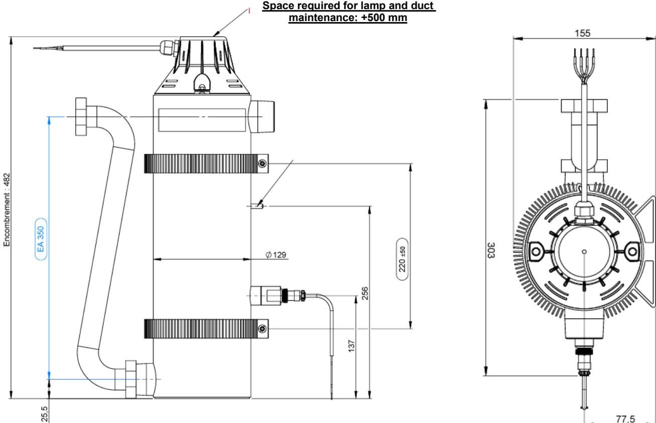
In the treatment chamber, the UV lamp is placed in a quartz sheath. This achievement prevents the lamp from cooling down by the passage of water, as its maximum efficiency is at 40°C. The layer of air between the duct and the lamp is sufficient to maintain this temperature: the quartz duct serves as a separation between the lamp and the liquid as electrical and thermal insulation.
