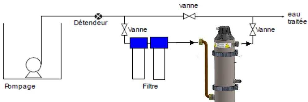
**It is imperative to always position the water inlet on the lowest tap of the reactor => filling by low point, outlet by high point, to evacuate air accumulations**
